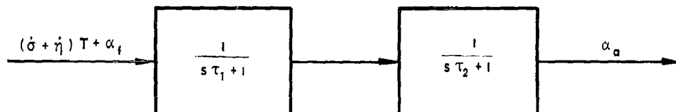
FIGURE 7-15. EFFECT OF FILTERING ON INPUT AZIMUTHAL RATES
