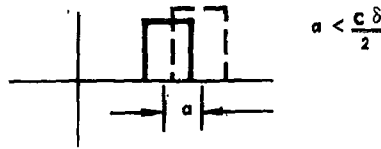
FIGURE 4-6. RECEIVED PULSE OVERLAP
